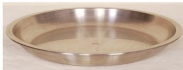
The stainless tray for Unipod comes 20 inches in diameter and 3 inches deep. The tray is formed out of high quality, rustproof 310 stainless sheeting, which has been spun on a lathe to create a beautiful rounded shape. The edge of the tray has a rounded lip, which adds both strength and aesthetic appeal to the tray and stand. There's a hole drilled at the center of the tray for mounting the tray onto the stem of the stand.
