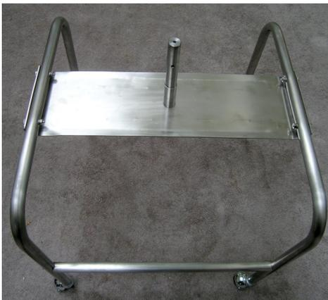
The legs of the base/floor stand are held together by a solid stainless cross plate. At the center of this plate is a solid stainless stub for mounting the top. The catch tray slides over this mounting stub to rest on top of the base. Once the tray is in place, the stem and top also slide onto this mounting stub. A stainless hex bolt fits through a hole at the bottom of the stem and into a threaded hole in the mounting stub to lock the stem/top securely to the base.
